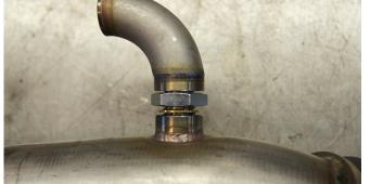
Thread the spacer as far as you can into the bung while still leaving room to orient the end for installation of the O2 sensor. With the spacer oriented properly, tighten the jam nut down. Thread the O2 sensor into the spacer. Make sure O2 sensor wiring is properly secured.
